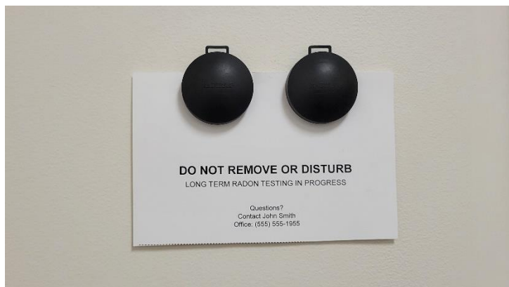
Pictured above are two radon testing devices as they may be deployed around Naval Support Activity Naples.
